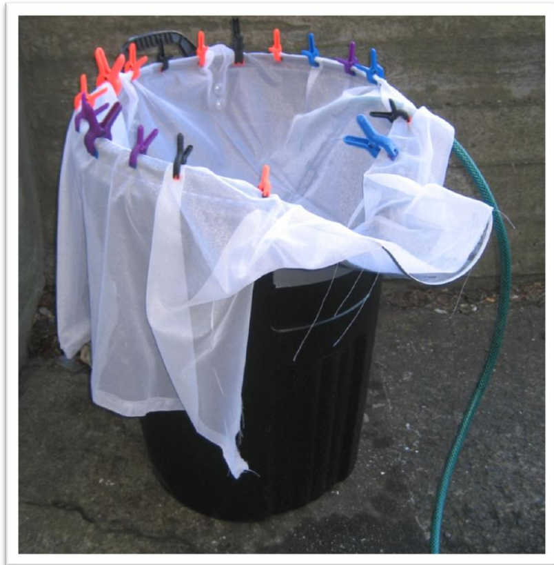
Fig. 1: Constructed flotation unit.
